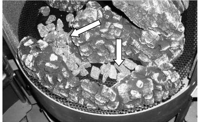
7. Sprinkle the charcoal embers over the burner ports only. Ensure that you leave the ports open over the pilot and where the main burner ignites.
