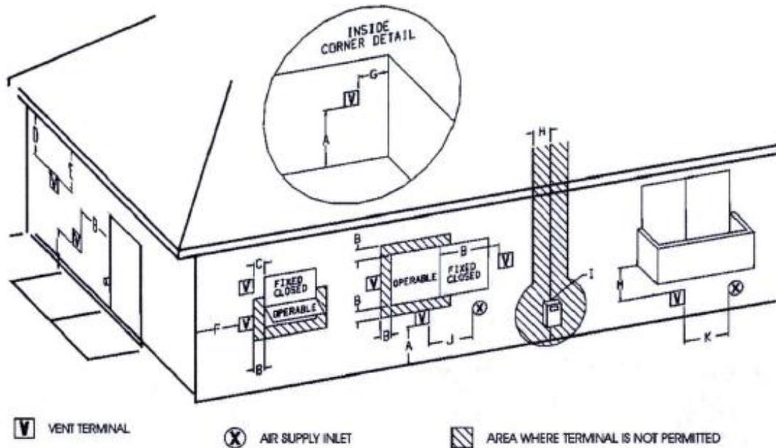
**Figure 5: Termination Location & Clearances**
